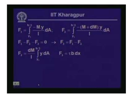
Likewise the value of  $F_2$  = Integral<sub>y1</sub> to the power of h/2 - (M + dM) (Y)/I (dA)
