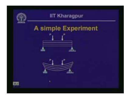
Let us evaluate what is the magnitude of the shearing stress in terms of the sectional parameters. Before we really go into the evaluation of the shearing stress, you can think of a small experiment. Take a number of small beams which are supported on supports and these beams individually are racing one after another. We apply a load on to the top of this particular beam and it is expected that it is undergoing deformation in this particular format as it is shown over here.
