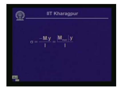
What is the impact of bending stress in arriving at a size of a beam? Last time, we had discussed that the flexible formula or the bending formula is given by this particular expression that Sigma = -MY/I. As you know M is the bending moment, Y is the point at which we are trying to evaluate the stress and the distance from the neutral axis; 'I' is the moment of inertia.
