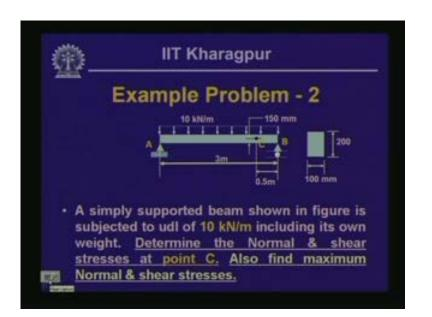
Take the example which corresponds to the one which we have discussed. The example deals with the aspects of shear stress that a simply supported beam is subjected to on a uniformly distributed load of 10 kNm including its own weight. Determine the normal and shear stress at point C and at this particular point, we will have to find out the value of the normal stress which is generated due to bending and the value of the shear stress.
