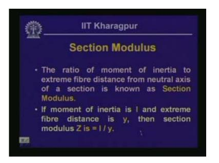
In fact, we have said that Z is a parameter which is I/Y and this is what we call section modulus. The ratio of moment of inertia of section to the extreme fiber distance from the neutral axis of the section is known as the section modulus. If I is the moment of inertia and  $Y_{max}$  is the extreme distance from the neutral axis of the out of fiber then I/Y<sub>max</sub> = Z.
