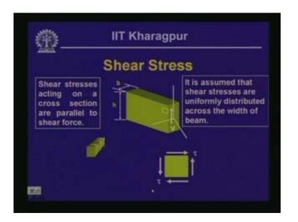
In the previous two lessons we have computed the values of the bending stress. That means when beam members are subjected to a stress result which is a bending moment for that we could evaluate the value of the normal stress because of such a bending. As you have noticed that when beam members are subjected to loads, not only are they subjected to a bending moment but at location they are subjected to shear forces.
