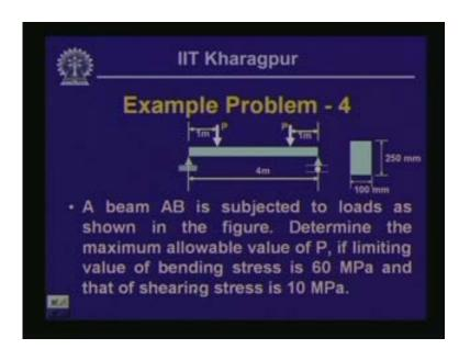
There is another problem where a beam is subjected to two concentrated loads and you have to compute the maximum value of b so that the bending stress does not exit 60 MPa and shearing stress does not exit 10 Mpa. We will look into this particular problem next time.
