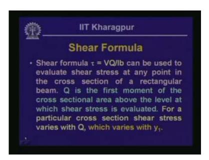
From this particular shear formula which we have just derived, we find that the expression for the shearing stress Tao = VQ/Ib and this can be used to evaluate shear stress at any point in the cross section of a rectangular beam. A rectangular beam is a beam having a rectangular cross section. The term Q is the first moment of the cross sectional area above the level at which we are looking for the shear stress and for a particular section.
