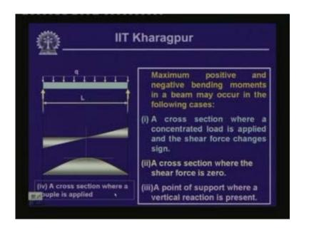
The maximum bending point may occur at a support point where you have a vertical reaction and a cross section where a moment is present. These are the situations where you can expect that the value of the bending moment could be maximum at those points. This could be positive maximum or a negative maximum. We talked about the magnitude of the bending moment where it could be on the negative side as well as the positive side.
