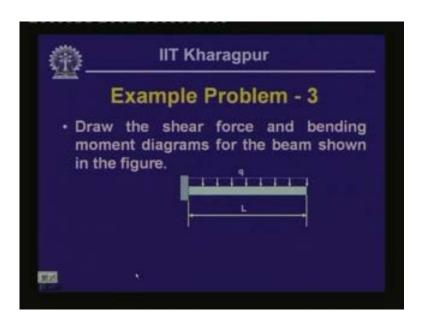
Let us look into another kind of beam. As you can recognize that this particular beam is supported at this edge; edge A and end B. End B is unsupported or free and we have defined this kind of beam which is supported at one end and free at the other as a cantilever beam and this particular cantilever beam is subjected to a uniformly distributed load.
