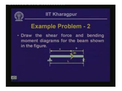
If we take the moment of all the forces with respect to 'a' and if we say that the moment with respect to a = 0 then we have  $R_B$  (L) which is in the anti-clockwise form. Also we have the concentrated moment which acts in an anti-clockwise manner,  $L + M_0 = 0$ . The value of the reactive force  $R_B = -M_0/L$ . Since RA + RB = 0, the value of the reactive force  $R_A = R_B = L + M_0 / L$ .
