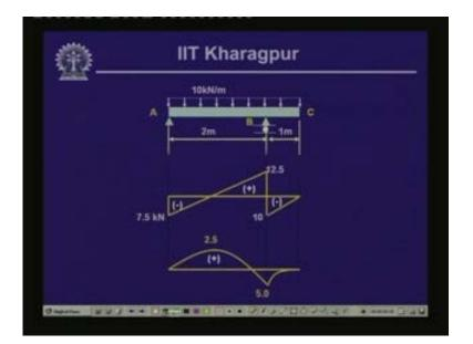
Let us draw the shear force and bending moment diagram where the sheer force is 7.5kN. At this particular point, since we have the overhang beyond this, it changes over to 12.5 and from 12.5 to reactive values here, it changes down to -10 and finally 0 over here. This is the shear force diagram for this particular beam and if we compute the bending moment we will find that the bending moment will vary again in a parabolic manner.
