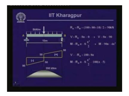
As you can observe from this bending moment diagram that at this particular point, the tangent to the bending moment diagram is a horizontal one. It indicates that the derivative at that point dM/dX is 0. Corresponding to this, as you can see the shear force at this particular point is 0. Let
