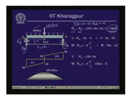
Let us suppose that we cut the beam at this location. Let us say this is 'a a' and take the free body of this particular part then we have the reactive force  $R_A$  over here. We have the distributed load which is at 8 kN per meter. We have the shear force P and the bending moment M at this cut section. If we take the vertical equilibrium, the equilibrium of the vertical forces then V +  $R_A$  are in the same direction - 8 kN per meter.
