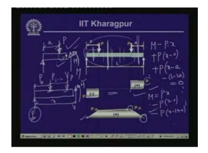
Let us look at another example where we have a concentrated moment. We have to draw the shear force and the bending moment diagram for this particular beam where we have a concentrated moment which is at a distance of A from the left hand A this is B and the span of the beam or the length of the beam is = L. As we have seen earlier, this is supported on a hinge and this is supported on a roller.
