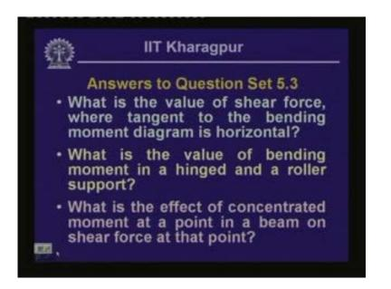
What is the value of a bending moment in a hinged and a roller support? This question is straightforward as we have seen while evaluating the reactive forces at the hinged support and the roller support. In the case of a hinged support it is constrained to move against the horizontal and the vertical direction but it is allowed to rotate, thereby there is restriction on the rotation and thereby it cannot sustain any moment.
