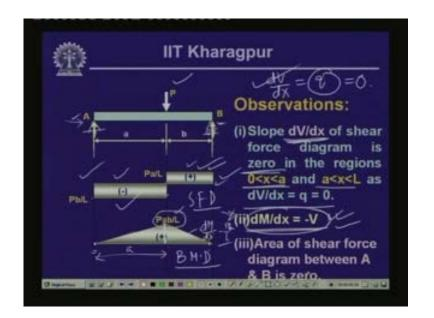
If we take the shear force diagram between these 2 points, this Pb/L which is negative multiplied by 'a'. This is -Pab/L and over this region we have Pa/L (p) which is plus. We have Pab/L plus and if we sum them up we get 0. Again this satisfies the condition that the area of shear force diagram between 'a' and b = 0 and these are the observations from this particular diagram.
