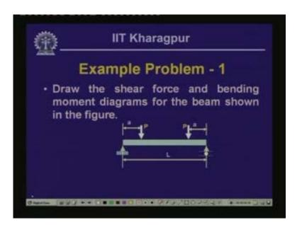
As we have done in the past, let us draw the free body diagram of the whole beam where we have a vertical reaction and a horizontal reaction. At the roller support, we have a vertical reaction and we call this as  $R_A$  and this as  $R_B$  for the beam a b and the horizontal force H is  $H_A$ . As we have seen in this particular beam the summation of horizontal force which is 0 gives us the values of  $H_A$  as = 0.
