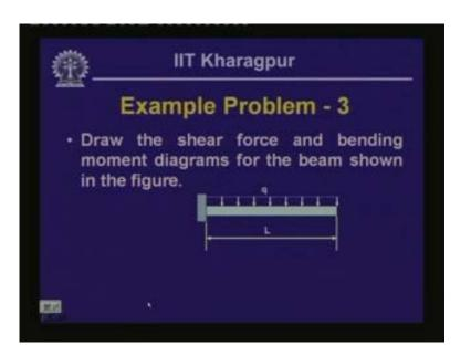
We will have to draw the shear force and the bending moment diagram for this particular beam. Let us draw the free body diagram of the whole beam and thereby let us compute the reactive forces first. The reactive forces are the vertical reactive force which is RA, the horizontal force which is  $H_A$  and a bending moment which is  $M_A$ .
