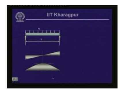
In the last lesson, we had seen that the differential equation dV/dx along the length of the beam is equal to q where V is the shear force and q is the uniformly distributed load. If we have q = 0 then what happens to V? Subsequently, if we take the differential of this moment dM/dX this is equal to - V. If the shear force V is 0 then we had said that dM/dX = 0 and over that particular zone moment is shown as a constant.
