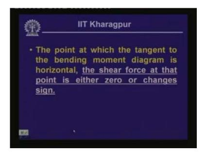
This is the consequence of the particular question. Now the answer to that question then is the point at which the tangent to the bending moment diagram is horizontal, the shear force at that point is either 0 or changes its sign. Let us look into the second question.
