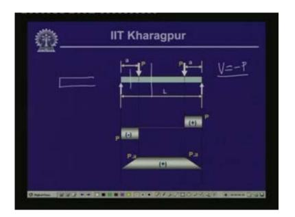
What happens to this diagram if we take the segment over here? As we have seen that on the left segments, on the segment 1 after taking the free body, we have V = -P. Let us take a segment here where there is a free body diagram and the free body diagram looks like this. (Refer Slide Time: 33:02 - 40:22) Here we have the reactive force  $R_A = p$ , we have the value of force P which is at a distance of 'a' and at this point we have the shear force and the bending moment as V and M.
