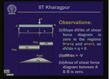
If you notice that the shear force and the bending moment diagram which we have plotted for a beam which is A B subjected to a concentrated load P at a distance of 'a' and this is on a hinged support and this on a roller support. Since there are no horizontal forces, we say h = 0 and we have these 2 vertical supports. Correspondingly, we have a shear force diagram and a bending moment diagram.
