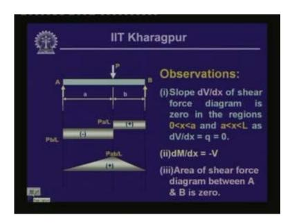
In the last lesson we had discussed the features of a shear force and bending moment diagram and how to plot them. We have defined a shear force and a bending moment diagram based on the example which we had seen last time both for the concentrated load, simply supported beam to a concentrated load or a simply supported beam subjected to a uniformly distributed load. Let us look into some of the salient features of shear force and the bending moment diagram.
