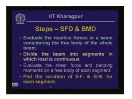
If we evaluate the shear force and bending moment on a free body of each segment and plot the variation of shear force and bending moment for each of such segments then we will get the shear force diagram and the bending moment diagram of that particular beam. These are the steps one has to go through to draw the shear force of the bending moment diagram.
