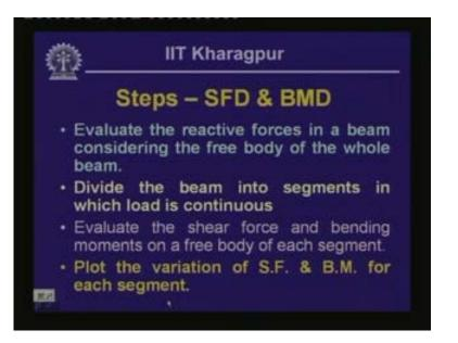
Having known these aspects of the bending moment and shear force diagram, we are in a position to summarize the steps necessary for drawing the shear force and the bending moment diagram. Given a beam with certain kinds of loading and support conditions, the reactive values of the supports should be such that they can be evaluated using the equation of Statics. That means they are statitically determinate systems.
