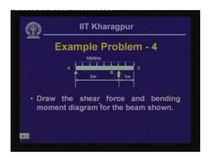
We have another example problem where we will have to draw the shear force and the bending moment diagram for this particular beam and exactly in the same way for the hinged support. We write down the reactive force  $R_A$ , the horizontal force  $H_A$  and the vertical force  $R_B$  and as you can recognize  $H_A = 0$ , we can compute  $R_A$  and  $R_B$  from the free body and then we can take segments to find out the values of shear force and bending moment.
