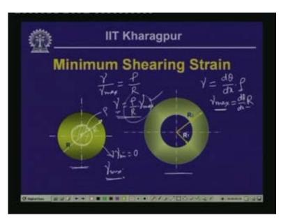
The third question was; what is the value of minimum shearing strain for solid shaft as well as for the tubular shaft?
