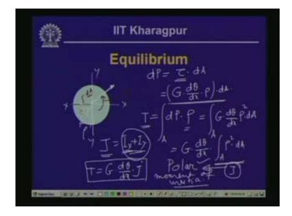
Now if we try to evaluate the rotation over the entire length of the bar, here the twisting moment which is applied in the bar is related to the rotation part in unit length in terms of the polar moment of inertia of the section and the shear modulus. If we like to find out that the bar which is fixed at one end and subjected to twisting moment on the other, what is the change in the angle or the change in rotation over the entire length of the bar?
