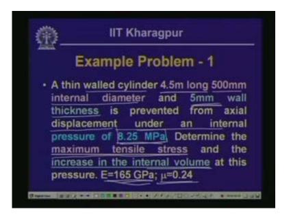
A thin-walled cylinder 4.5 meter long, 500 mm internal diameter, and 5 mm wall thickness is prevented from axial displacement under an internal pressure of 8.25 MPa. All we have to do is determine the maximum tensile strength and the increase in the internal volume at this pressure 8.25 MPa given the value of E is equal to 165 GPa and mu is equal to 0.24. Let us look into how you get the maximum tensile stress and then the change or increase in the internal volume.
