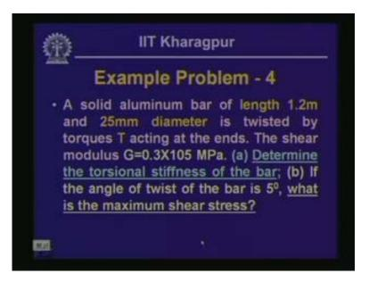
We have another example problem where a solid aluminum bar of length 1.2m and 25 mm diameter is twisted by torques T acting at the ends. The shear modulus is given and you will have to determine the torsional stiffness of the bar and secondly if the angle of twist of the bar is 5 degrees then what is the maximum shear stress?
