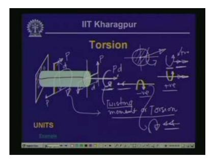
This is how it gets rotated when a twisting moment is applied on the bar which was initially straight. This is how it gets rotated. Here this end being fixed it moves and then forms an angle over here. This particular original radius is getting changed or there is an angular change over here, and this is what we will be looking into while deriving the formulae for torsion.
