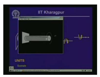
Coming to the units of moments here the unit of the force is Newton and the distance is written in meters. Hence the twisting moment or the torsional moment which you have has the unit Newton meter Nm.
