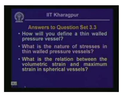
A thin-walled pressure vessel may be defined in this particular form. Basically, thin-walled pressure vessels are the closed pressurized containers and when these pressurized vessels are subjected to internal pressure they are subjected to stresses. We classify these pressure vessels as thin-walled pressure vessels. When the thickness of such a vessel is sufficiently small compared to the radius of the container the stresses are almost uniform throughout the thickness.
