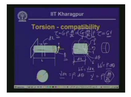
If you look into this particular figure, this is the radius vector here r and now at a distance of rho rho as considered in this particular configuration as rho, the shear stress is tau given by tau is equal to G  $\frac{d\theta}{dx}$ \* rho. Now when this one goes to the surface it becomes tau<sub>max</sub>, tau<sub>max</sub> is equal to G  $\frac{d\theta}{dx}$ r, when rho becomes r which is the maximum shear stress.
