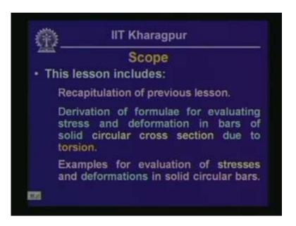
Also, one should be able to understand the concept of shear stress which gets generated due to torsion, and one should be in a position to evaluate stresses and deformation in solid circular bars which develop due to torsion.
