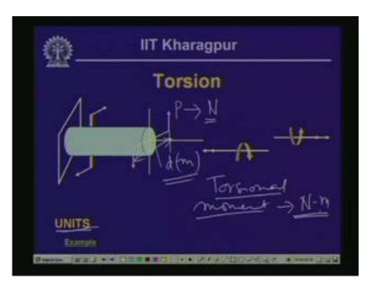
Let us look into this particular configuration which is again a solid circular bar, the cross-section is a circular one and it is solid. It does not have any hollowness in such a system. If this particular bar is subjected to a positive twisting moment then what happens to this particular system?
