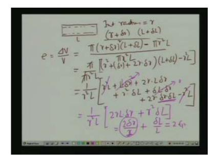
Now this is equal to  $2 \in 1+ \in 2$  so notice that  $\in 1$  is the strain in the circumferential direction and  $\in 2$  is the strain in the longitudinal direction.
