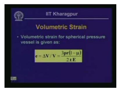
This is what is represented here that the value of the volumetric string e is equal to  $\frac{3pr(1-\mu)}{2t.E}$ .
