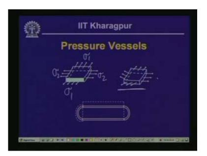
That means the stress or the pressure which is being exerted by the content of the spherical vessel is being resisted by the vessel in all directions. As we have seen in both the cases the cylindrical as well as the spherical vessel, the pressure which is exerted on the curved surface is normal to the surface. And since the wall is thin the variation of the stress across is negligibly small and we disregard that.
