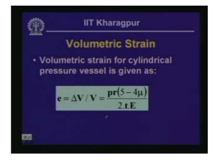
The  $\frac{\Delta V}{V}$  is equal to  $\frac{\text{pr}(5 - 4\mu)}{2.\text{t.E}}$  this is the volumetric strength in case of cylindrical pressure vessel now.
