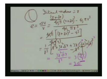
Now we can compute the value of e in terms of stresses and it comes as e is equal to  $3 \in$  and  $\in$  we can write in terms of sigma is equal to  $3\frac{(1-\mu)}{E}\sigma$ . And in case of spherical vessels sigma is equal to  $\frac{pr}{2t}$  is equal to  $\frac{3(1-\mu)}{E}\frac{pr}{2t}$  is equal to  $\frac{3(1-\mu)}{E}\frac{pr}{2t}$ .
