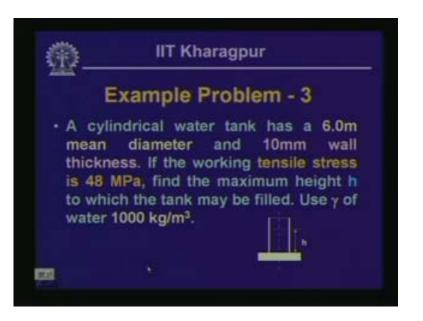
Let us look into the third example; a cylindrical water tank has a 6m diameter. Let us take this as our internal diameter only which is 6m as 6000 mm and the thickness of the tank wall is 10 mm. Now if the working tensile stress is 48 MPa the limiting stress on the vessel is 48 MPa, find the maximum height h to which the tank may be filled. Use  $\Gamma$  of water unit weight of water as 1000 kg/m cube.
