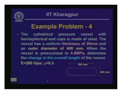
Let us look into another problem. Here we have a pressure vessel which is basically a cylindrical pressure vessel, this is the cylindrical part having 600 mm in length and is connected with a hemispherical end. The two ends are hemispherical having a diameter of 400 mm and the diameter of this particular hemispherical end is the external diameter. The cylindrical pressure vessel with hemispherical end caps is made of steel.
