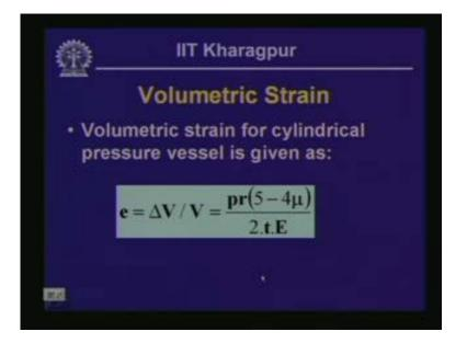
When you have a liquid inside a container whether it is a cylindrical or spherical vessel, it undergoes change in the diameter thus there is a change in the volume of the container. If a volume of a cylindrical or spherical vessel undergoes a change then we should be in a position to compute the changes in the volume.
