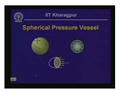
We had evaluated the values of the stresses. For a spherical system or the spherical vessel of this kind the stress that exists is sigma in both the x and y direction. The resistive force which is sigmaA is equal to 2pi rt where r is the internal radius of the sphere or spherical vessel and t is the thickness of this particular vessel.
