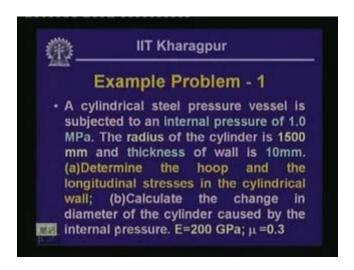
This was a cylindrical steel pressure vessel subjected to an internal pressure of 1 MPa, radius of the cylinder is 1500 mm and the thickness of wall is 10 mm. Last time we had computed the values of hoop stress which is the circumferential stress and the longitudinal stresses in the cylinder. Now we have calculated the change in the diameter of the cylinder which is being caused by this internal pressure.
