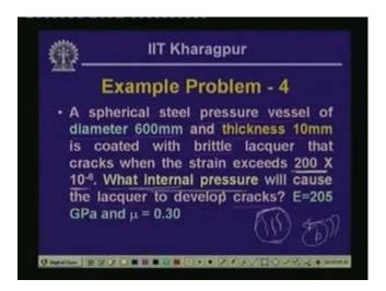
Now let us look into another example of a spherical ball or a spherical vessel where we have a spherical steel pressure vessel of diameter 600 mm and thickness 10 mm coated with a brittle lacquer and that cracks when the strain exceeds 200(10<sup>-6</sup>). What internal pressure will cause the lacquer to develop cracks?
