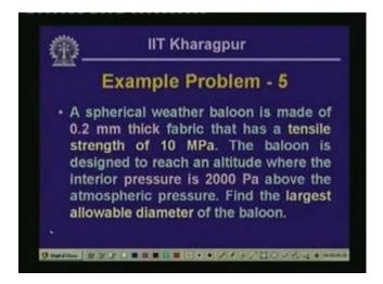
Let us look into another example of this particular category where we have the spherical vessels; a spherical weather balloon is made of 0.2 mm thickness fabric and that has a tensile strength of 10 MPa and the balloon is designed to
