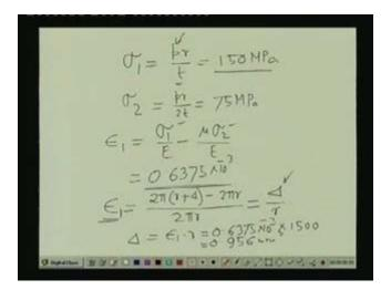
if you remember, the values which we had calculated last time was the value of  $\sigma_1 = \frac{pr}{t}$  and this we had computed as 150 MPa where p was 1 MPa, r was 1500 and t has a thickness of 10, we had the value of  $\sigma_1$  as 150 MPa and the value of  $\sigma_2$  which we had obtained was half of this which was  $\frac{pr}{2t} = 75$  MPa.
