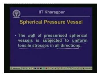
Therefore the wall of pressurized spherical vessels is subjected to uniform tensile stresses in all directions. As we have seen wherever we cut across in a spherical vessel we get the same kind of distribution and as we have equated the resistive force  $\sigma \times 2\pi rt$  is equal to the pressure exerted by the content multiplied by the
