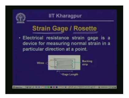
This is the configuration of the strain gage as shown here where this particular area is the backing strip over which the wire is placed and this is the gage length of the strain gage. Various sizes of the strain gages are available, they range between 2 mm to even 40 mm to 50 mm size.
