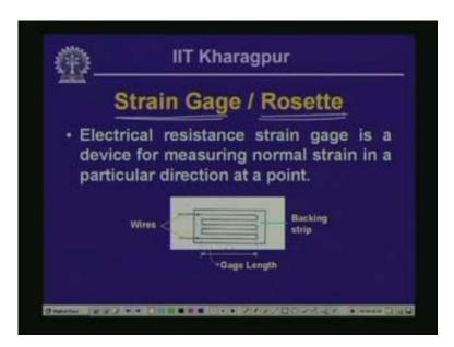
Having looked into these questions now let us look into the aspects which we are going to discuss today: the concept of the strain gage and consequently the term which is called as Strain Rosette. Many a times what we need to do is that experimentally we need to measure the strain at a point in a stressed body and that can be done using a device which we call as Strain Gage.
