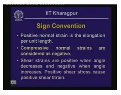
Now, as we have evaluated the strain at a point, if the reference axis is oriented at an angle of theta with reference to the rectangular axis system x and y we have seen how to compute the value of the maximum normal strain which we have called as the principal strain, we have see how to compute the value of the maximum shearing strain and the orientations of the principal strain and shearing strain through the angles theta<sub>p</sub> and theta<sub>s</sub>.
