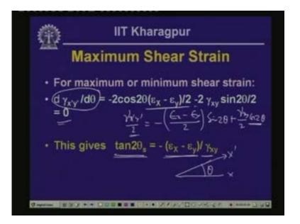
As we have seen the shearing strain at any orientation which is oriented at an angle of theta with reference to x axis which is our x prime gamma x prime y prime corresponding to that particular direction is  $epsilon_x$  minus  $epsilon_y$  by 2 cos 2theta plus  $gamma_{xy}$  by 2 sin 2theta plus  $gamma_{xy}$  by 2 cos 2theta.
