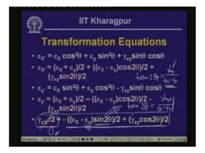
Here if you look into the shearing strain gamma x prime y prime is given as this, now we have already looked into the angle at which the maximum normal strain occurs is  $tan(2theta_p)$  equal to gamma<sub>xy</sub> by epsilon<sub>x</sub> minus epsilon<sub>y</sub>.
