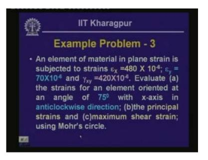
The next example is that an element of material in plane strain is subjected to strains of these. We got to evaluate the principal strain and the shear strains and also strain at an angle of 75 degrees.
