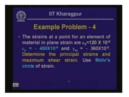
The fourth problem is that the strain at a point for an element is given by these values. We will have to determine the principal strain and maximum shear strain using Mohr's circle of strain.
