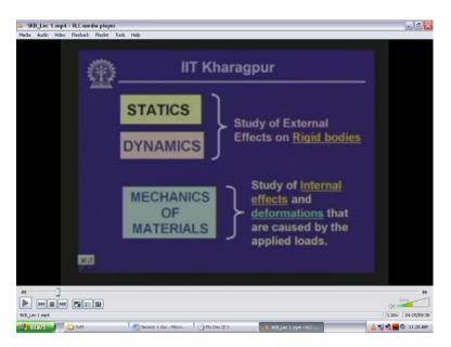
In fact we look into what we mean by design. When we try to arrive at a particular size of the member, we need to know how much it deforms and what is the effect of external load on that member internally and these aspects are dealt in the particular subject, which we call mechanics of the material.
