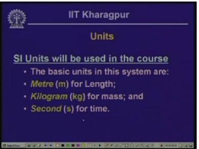
When we talk about the numerical problems or the algebraic problems, we talk about the units and the basic units which are used. We use the international system of units in this particular course. And the basic units for these in the international system are
