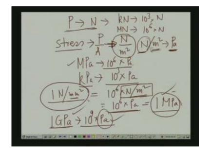
Also many a time, we use parameters as we have seen Force, which we define in Newton, it could be in kilo Newton or mega Newton, which is 10 to the power 3 Newton or 10 to the power 6 Newton. And we define another parameter, which we call as stress in few minutes. This unit for stress or the stress we define as the force per unit area. So as we have defined, the unit of force is Newton and area is m square. So the unit for stress we call N by m square and this is called as Pascal, Pa.
