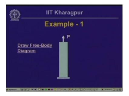
Now in this example we are interested to draw the free body diagram for this. Now this is the part which is subjected to a tensile pull. Now if you would like to draw the free body diagram of the whole part then, the free body diagram will be like this: that it is acting on by this force
