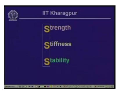
So now we are in fact in Strength of Materials, we are interested in these three characteristics: first one is strength, another is stiffness and another is stability and these are called as three Ss of strength of material. So we are concerned with the three Ss: parameter strength, stiffness and stability.
