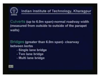
For culverts up to 6 m span the normal roadway width is maintained and is measured from outside to outside of the parapet walls. In case of bridges where the span is greater than 6 m the clearway between kerbs depend on whether it is a single lane bridge or a two lane bridge or a multi-lane bridge. Again the prescribed or the recommended widths in each of these cases are available in Indian Roads Congress guideline. So you may refer to appropriate IRC code for obtaining the recommended values.
