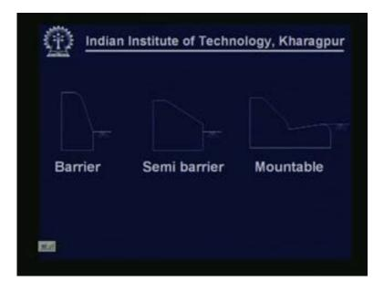
There are different shapes of kerb as shown here: barrier type kerb, semi-barrier type kerb and mountable kerb. Mountable kerbs are provided where we want the vehicle to cross the kerb with very minimum difficulty. Yes, there is kerb, there is a barrier but vehicle can easily cross that barrier. So wherever we feel that there should be provisions for vehicle to cross the barrier easily there we use mountable kerbs.
