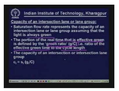
Now the capacity of an intersection lane or lane group may be calculated now easily. Remember that the saturation flow rate represents the capacity of the intersection lane or lane group assuming that the light is always green. But this is not the case in reality. The light is not always green so the portion of the real time that is the effective green is defined by the green ratio.
