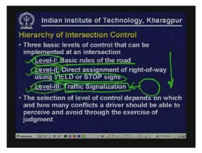
Further we shall move to Traffic Signalization. We have Levels 1, 2 and 3. The selection of level on control depends on which and how many conflicts a driver should be able to perceive and avoid through the exercise of judgment. So like I said, carefully observe this part. What type of
