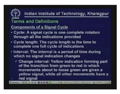
First is the component related Signal cycle. What exactly is Signal cycle? A signal cycle is one which has complete rotation through all the indications provided. You are familiar with traffic signals? If you are moving sometimes, it is red, amber or green. So a complete rotation through all the indication is provided by the signal cycle.
