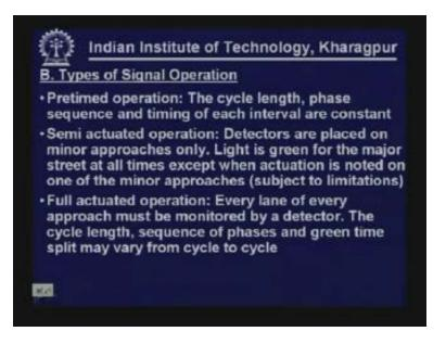
Now coming to signal operation there are three types of operation such as pretimed operation, semi actuated operation and full actuated operation.
