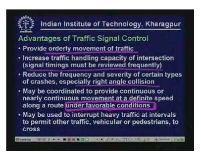
Signals may be used to interrupt heavy traffic at intervals to permit other traffic, both vehicular and pedestrians to cross. In some cases you may find heavy traffic and small vehicles moving and it is not safe to cross. So you intermittently wait so that other vehicles or pedestrians can cross efficiently and safely.
