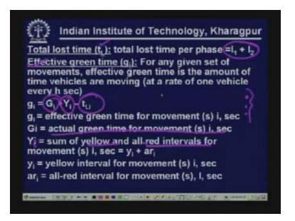
Now we have the total lost time. This is basically the start-up lost time plus the clearance lost time. So it is 11 + 12 and (......45:21).
