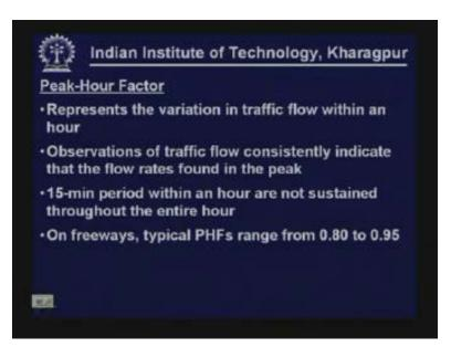
Peak-hour factor is basically to represent the variation of traffic flow within an hour.
