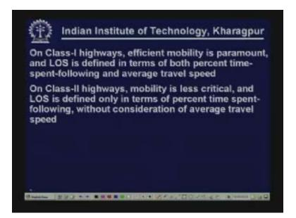
On class II highways the mobility is less critical and therefore LOS is defined only in terms of percent time spent following without consideration of average travel speed. So that is why LOS is different, the measure of effectiveness is different on the class I and class II type two-lane highways.
