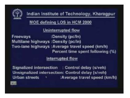
Let us have a look at some of the measure of effectiveness for different LoS for uninterrupted flow facilities and also for interrupted flow facilities. For uninterrupted flow facilities say freeways the measure of effectiveness is density. For different facilities different measure of effectiveness are defined. For freeways it is density which is normally expressed as passenger car per lane. How many passenger cars per lane, per kilometer?
