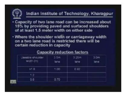
The capacity of two-lane road can be increased about 15% by providing paved and surface shoulder of at least 1.5m width on either side. This is again an IRC provision. So you provide paved and surface shoulders of at least 1.5m width on either side then the capacity of the service volume values may be increased by 15%.
