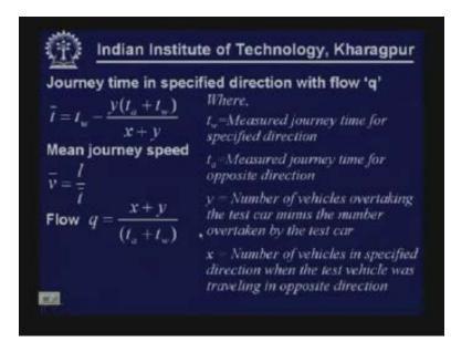
Now we record a number of data here and the travel time in each direction separately and for each direction of travel the number of overtaking vehicle, the number of overtaken vehicle and number of vehicles from opposite directions etc are recorded and then appropriately they are adjusted to calculate the average speed or the representative stream speed time and once we calculate the ..... 55:23 using the appropriate calculations then you can calculate V and Q.
