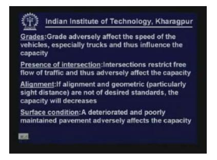
Grade: also affects the speed of vehicle particularly if you have substantial proportions of commercial vehicles or heavy vehicles. Therefore on grades the presence of heavy vehicles together may really influence the capacity to a large extent.
