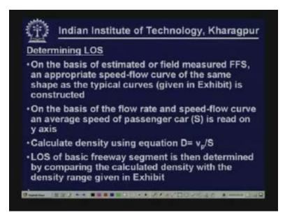
Now determining LOS we estimated field measured free flow speed so we have mentioned how we can calculate FFS and the appropriate free flow curve of the same shape of the typical curves is constructed then on the basis of the flow rate and the speed of curve and the average speed of the passenger car is read on the y axis.
