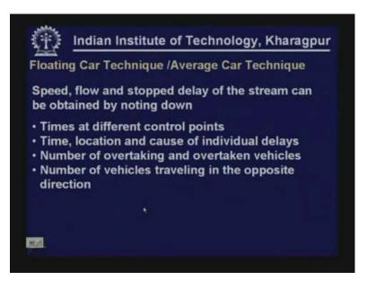
A little bit further discussion on floating curve technique or average car technique these two are almost equal. Only in one case the overtaking and overtaken vehicle are made equal but in the other case they may vary. In floating car technique or average car technique speed, flow and stop delay of the stream can be obtained by noting down the following;
