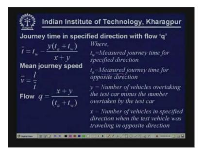
Similarly when the test car is traveling towards south again we note down the overtaking vehicle, overtaken vehicle which is coming from the opposite directions so all this data are required. From the recorded data from multiple runs we calculate the journey time and specified average journey time in a specified direction with the flow queue, how the flow is calculated? Flow is X + Y by Ta + Tw. What is Ta? Ta is measured journey time for opposite direction.
