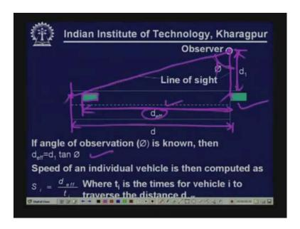
There could be errors due to early or late depressing of stop watch but this tends to be random so it can be minimized or it cancels out. Of course this error can be minimized using longer trap length because if the travel time is more the percentage error will be less. But obviously we cannot make it too longer then the meaning of spot speed will be lost.
