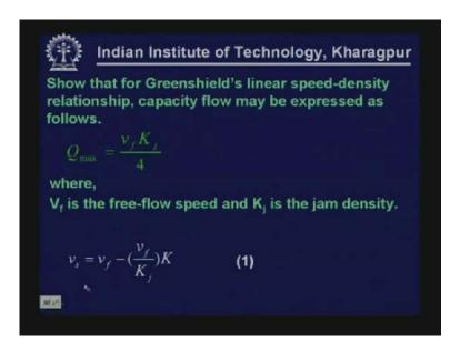
Show that Greenshield's linear speed density relationship and prove that Qf = Vf into Kj by 4 so this is the linear relationship given by Greenshield.
