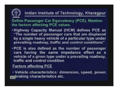
For PCE you can know that mixed vehicle we tried to express the simple vehicle type using the concept of PCU. It is the number of passenger cars having the same impedance effect as a vehicle of a given type under a prevailing road way traffic and control condition. There are factors which are affecting PCE vehicle characteristics as follows:
