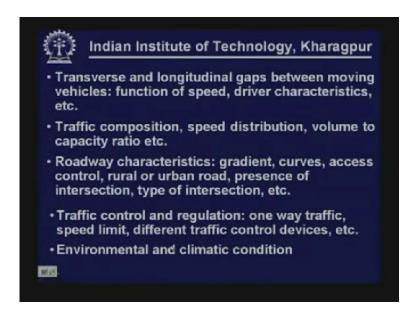
Transverse and longitudinal gaps, traffic composition, speed distribution, volume to capacity ratio, roadway characteristics, geometrics like gradient, curves, access control, etc, then we have traffic control and regulation and environmental and climatic condition.
