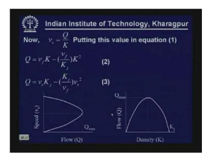
If you use Vs = Q by K that is flow equal to speed into density then you can get equation 2 and 3, you can express Q in terms of K and Q in terms of speed. So take that derivative dQ dK = 0 which will give you the k value at capacity and make dQ dV = 0 that will give you V value at capacity so at maximum flow or capacity Vm into Km which is nothing but Vf into Kj by 4, thank you.
