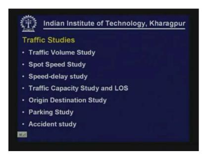
There are several types of traffic studies that are carried out including traffic volume study, speed study and within the speed study also spot speed study, speed and delay study, traffic capacity study and level of service, origin destination study, parking study, accident study and there are so many other kinds of specialized traffic studies. They are all different types of studies which are required to be carried out for specific purposes.
