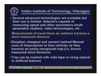
Several advanced techniques are available but remember that again their use is limited because of the cost considerations. Detectors capable of measuring speed and other parameters they are available which are normally used for multi parametric studies, video technologies are available which are used for volume counts, speed measurement and so many other things but again cost is a major consideration for wide spread applications of these advanced technologies for common type of statistics.
