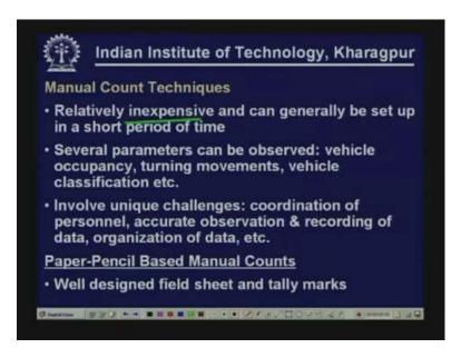
First coming to manual count techniques: manual count techniques as I mentioned they are relatively inexpensive, it can generally be set up in a short period of time, you can quickly set up count techniques. These are the major two advantages for which we go for manual counts. There are other advantages also like several parameters can be observed which for automatic or
