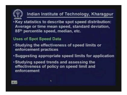
When it is the distribution speed is distributed following certain distribution. So when it is distribution some key statistics are required to describe spot speed distributions. What are the key statistics that are normally used? Average or time mean speed, average observations over time, standard deviation, eighty fifth percentile speed, median value etc are the key statistics which are used to describe spot speed distribution.
