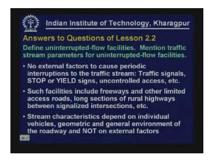
Quickly trying to answer the questions of lesson two point two; uninterrupted flow facilities is basically where there is no external factor. This is what we call as uninterrupted flow facilities.
