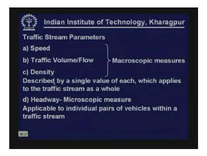
The stream parameters are macroscopic parameters and microscopic parameters both are used. Speed, traffic volume, flow and density are in the macroscopic parameter and headway is the microscopic parameter.
