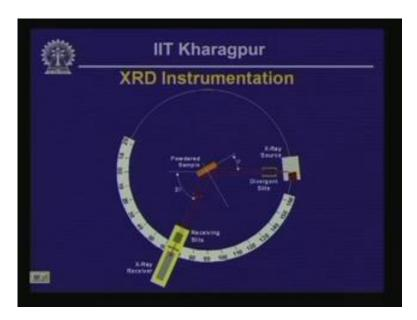
A schematic of an XRD instrument, X-ray diffraction instrument is shown on this cartoon here and you can see here what we have got is an X-ray source that actually made to impinge on a powdered sample, powdered crystal sample and then we have got a receiver that we can move actually along this graduated scale and we can note the intensity of the signal that is coming out of the powdered sample.
