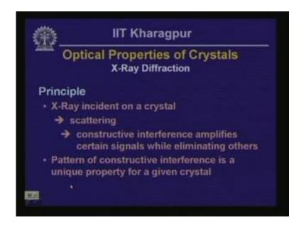
Now, we are going to actually consider another tool that is used to distinguish optical properties of crystals and that is X-ray diffraction. What is done in this case is X-ray is made to incident, X-ray is x-impinged on a sample of powder crystals and because of the regular distribution of the atoms in the body of the crystal, of the powdered material; there will be a scattering.
