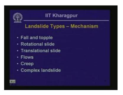
Then there could be other types of landslide classification, and this typing adhere looks at the mechanism that triggers the landslide. So, landslide could be classified as a fall or a topple. There could be a rotational slide. There could be a translational slide. Then there could be flows, creep and complex landslide. A complex landslide is really a combination of more than one of the types that precedes in the list, okay. So, let us look at what are these things one by one.
