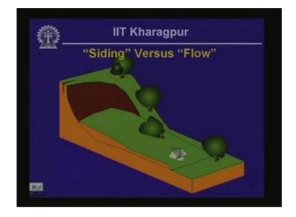
If you recall, sliding is of this type; in this case typically the movement is relatively slower, and the movement does not proceed to a great distance. Whereas in case of flow, the soil becomes liquid like or the failure mass becomes like a liquid, and you can realize
