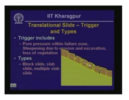
This is an illustration cross section really of the illustrating the process of block sliding. So, here what you see is pieces of rock, they are mobilized down slope near the slope face. This type of slide is called block slide.
