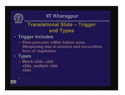
Trigger and types of translational slide, how translational slides could be triggered? They could be due to pore or pressure increase or steepening or increase of driving force because of a construction near the top of the failure surface or because of loss of vegetation as we looked when we are considering the rotational slides. Now types of translational slides include block slide, slab slide or multiple slab slide. What are these? We are going to come to that in the next little bit.
