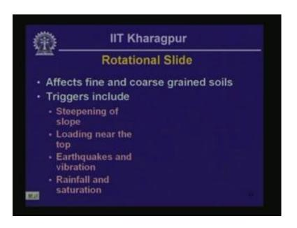
Rotational landslide, these types of landslide typically affect fine or coarse grain soils not so much; they do not occur so much in rocks. They are triggered because of steepening of slope, loading near the top, earthquakes and vibrations, and rainfall and saturation. How these mechanisms cause the landslide to get initiated. We are going to look at that in the next little bit, but before that lets look at the features of rotational landslide.
