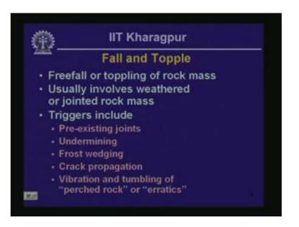
Fall and topple, what it means is that it involves free fall or toppling of rock mass; usually, this involves weathered or jointed rock mass. This type of landslide could be extremely fast, and this is triggered because of pre-existing joints undermining frost wedging, crack propagation, vibration and tumbling of perched rock or erratics. We are going to look at each of these things one by one, and some of them are explained in the cartoons that are going to come now.
