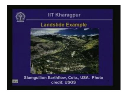
A few pictures I am going to quickly go through these pictures. This is a picture of Slumgullion earth flow in Colorado, United States. This is actually the flow characteristic is quite obvious from the failure mass which is visible here near the middle of this particular picture.
