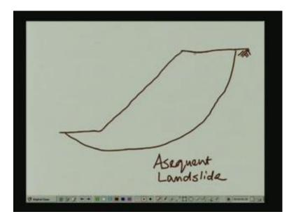
In this case, let us consider a slope in clay where there are no cracks or lenses or soft lenses or weak lenses through which the landslide can progress; it is a deposit of massive clay. In this case, often what happens? The failure surface takes the shape of a circle, and this type of landslide is going to be called an asequent landslide.
