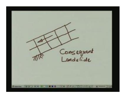
So, let us say you have got a slope where there are joint sets like this. This is a schematic picture of a cross section run through a particular slope, and the material underneath this jointed rock is massive and quite stable. And if this rock slides down slope in this manner, then this particular landslide is going to be called a consequent landslide, okay. So, then let us go and look at the other extreme.
