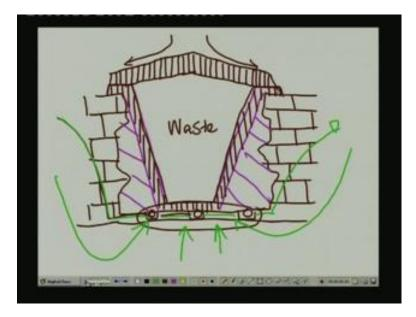
So, what we had there is an excavation within bedrock. This was, in fact, an original limestone quarry which got depleted got passed its economic use and then a landfill was constructed inside this particular quarry site, okay. Now if you recall what we had was a series of pipes at the bottom of the quarry itself. So, what these pipes do is to draw the groundwater table down to a configuration like this. So, let me use a different color pen.
