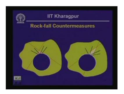
Now, another case which is the case involving involving a squid orientation of the wedge. Now here as I have indicated that the wedge is not always going to be unstable. You have to assess first whether the wedge is going to be stable or unstable. If you decide that the wedge is going to be unstable, then you can install rock bolts in order to stabilize this particular wedge from falling into the tunnel opening, okay.
