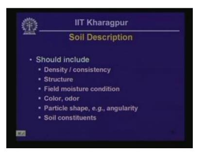
Now, soil description; you have to describe the subsurface units that are encounter during the investigation process. Now, soil description should include all those things; density or consistency, structure, field moisture condition, color or odor, particle shape such as angularity and soil constituents - whether it is composed of sand or whether it is composed of clay or whatever.
