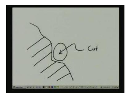
So instead of that, what we also learned earlier is that a preferable orientation of joint set would be like this. So, if the joints were to be orientated like this, then if we have got a steep cut at this location, then the cut is going to be relatively more stable. So, these considerations are verified from having a well laid out investigation, subsurface investigation land.
