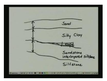
Now, underneath the silty clay, there could be a sand stone bed rock which could be interlayered with, interlayered, say siltstone and underneath the sand stone layer, there could be a silt stone layer. So, in a subsurface, from subsurface investigation, what we want to find is we want to actually find the sequence of these subsurface units that are going to be underlained, that are going to be below underneath a particular site.
