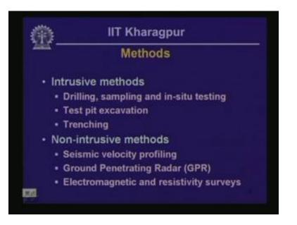
Now, we look at the different types of methods, different methods that we normally use, that are normally used in subsurface investigation. So, one class of methods that involves actually inserting a probe or getting or intruding into the subsurface layers. So, this type of investigation is called the intrusive methods.
