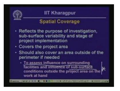
So, you saw there that we not only need to investigate along the proposed alignment of the highway, we also investigated laterally a little bit further out from the center line of the highway. So, that is what is meant in the last in the last particular point here; so you should take a note of this particular aspect as well.
