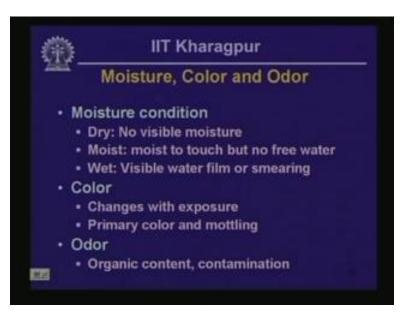
Then you have to describe moisture color and odor of a particular soil deposit. Moisture condition could be dry to wet. Dry means there is no visible moisture, moist means the deposit is moist to touch but there is no free water and wet means there is free water, free water film present on the surfaces of the individual particles.
