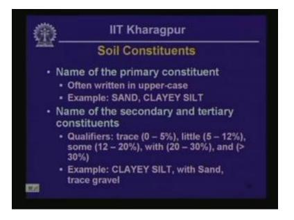
Then finally, you have to name the soil constituent; here you have to name the primary constituent of the soil and this includes say for example sand or clayey silt. And, you also have to name the secondary or tertiary soil constituent, secondary or tertiary soil constituent; so here you use qualifiers such as trace, little, some, with or and.
