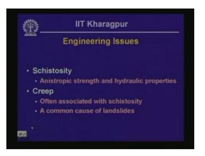
Engineering issues of metamorphic rocks includes schistosity and or foliation really and that leads to anisotropic strength development and hydraulic properties and often this type of rock exhibit creep behaviour and this actually leads to many landslide events.
