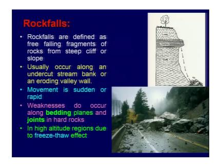
Coming to fall, the rock fall are defined as free falling fragments of rocks earth blocks from the steep cliff or slope usually occur along an undercut stream bank or an eroding valley walls. Movement is sudden or rapid weakness to occur along the bedding planes or joints in the hard rocks in high altitude regions this will take place because of freezing and thaw effect.
