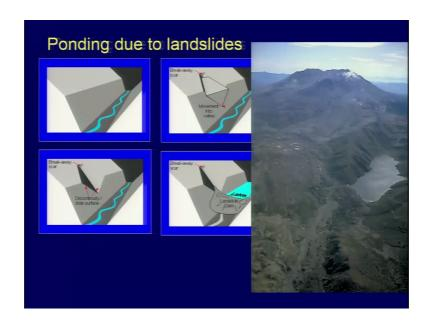
So, we also say landslide bank and this is an example of the typical lake formation along the valley, because of the landslide blocking the flow of the river.
