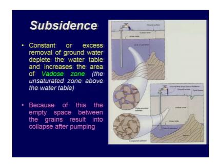
Another example is your excess removal of groundwater can also result into the subsidence. Now this example what has been shown here so, we have an round surface here vadose zone and in zone of saturation and then bedrock. So, if you keep on a removing excess water from this region which has been pumped out here, then the pore space which were relieved and filled by how this zone of saturation the pore space filled by water will go into compaction.
