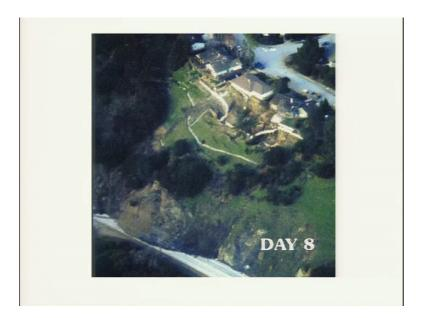
So, the landslip took almost like a week and there is an movie from US which shows the mass moment and you can see the top scars which have been developing here the extensional cracks and the mass which are moving down here in the toe is under the formation.
