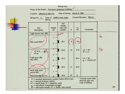
Now look at here, this is a boring data bore log or boring log we generally called boring log. How it is name of the project 2 story apartment building locations date of boring march 2 1982? Boring number 3; that means, earlier there are also 1 2 boring. Type of boring, hollow stem auger, how you use it by means of forward boring it has been done by means of mechanical. Or you have done by means of drilling machines; ground
