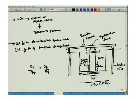
It has been carried out with a pit, with a pit it either circular or square plates. Square plates of size 300 mm to 700 mm.
