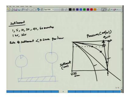
So, settlement you have to record it. Settlement record means each load increment, what settlement you are going to record, it may be 1 minute, 5 minute, 10 minute, 20 minute, 40 minute, 60 minutes. Then 1 hour, 2 hour like this we record settlements, then where
