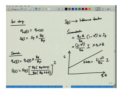
Actual real foundation equal to q u of your p, ultimate capacity of your plate. From plate load test I am getting pressure versus settlement from here, I am getting ultimate load of your plate.
