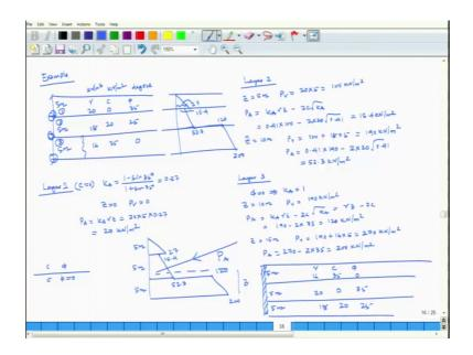
This is the case has been given. 5 meter, 5 meter, 5 meter, 3 layers are there. So, let us put it this is layer 1 this is layer 2 this is layer 3. And the properties has been given gamma C and phi. This is your kilo Newton per meter cube; this is your kilo Newton per meter square, phi in degree. For layer 1 it is 20, C is equal to 0, phi is equal to 35; that means, it is a cohesion less soil, for layer 2 it is 18, C is given 20 phi is equal to 25.
