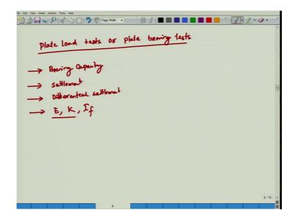
Let me start one of the field test program that is your plate bearing test. Plate load test or called plate bearing test. So, plate bearing test what you are suppose to get. You are supposed to get bearing capacity, settlement, differential settlement, E sub grade modules K. Then influence factor, these are all parameter you are suppose to get with a single test plate bearing test, there are scale effect.
