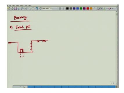
So, if I go this boring, first one as I said, it is the trail pit. Trail pit, in this trail pit generally make a pit of one meter by one meter by one meter. Then push this sampler tubes. This sampler tubes inside the ground surface; that means, this sampler tubes has to be pushed inside the pit. Remember it has to be pushed not it as not going to be hammer.
