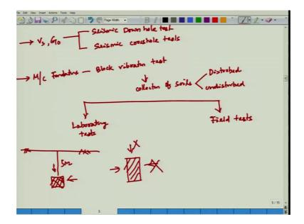
Then dynamic properties 0 velocity, vs 0 velocity vs, low stream shear modules g 0, seismic down hole test. Seismic cross hole test, then your machine foundations. For machine foundations, block vibration test. It if I make it into 2 components particularly geo technically investigations and subsoil explorations, I can say it first one is your collection of soils earlier I have say either it is disturbed or undisturbed.
