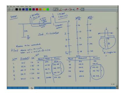
There is a building in that building one interior column, then another one is your exterior wall, dead load live load is given. There are 2 bore hole data, bore hole 1 is nearby from the interior column bore hole 2 is nearby from your exterior wall. And this design has been made and nothing has been assumed. We design considering where we are getting a consistent value of SPTN from the cumulative average.
