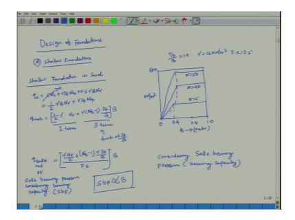
So, shallow foundation in sand we are considering safe bearing pressure considering bearing capacity as well as soil bearing pressure considering settlement, and from there for a residential building 25 mm settlement industrial building 50 mm settlement. So, allowable soil pressure is you kilo Newton per meter square. And it has come with your 10.5 N as well as 21 N.
