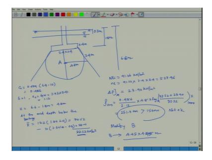
Settlement calculations, this is your ground water ground level. And there is a water table here. And this length is your 0.3 meter, and there is a footing here. And the size of the footing is this is your 2.4 by 2.4 meter. And this is your 0.4 meter. And this part is your 1.8 meter, and total will be your 6 point sorry here it will be your total from here to here from here to here total is your 6.5 meter.
