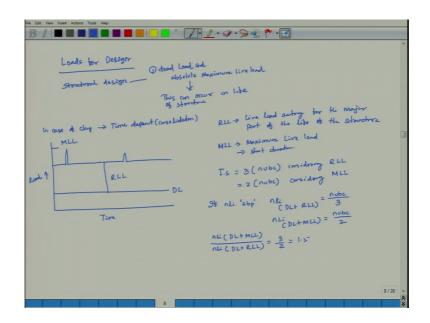
So, for structural design, structural design generally we take it, dead load, dead load and it is your maximum dead load and absolute maximum live load. So, structural design we are considering dead loads and absolute maximum live load, it will look at here. This can occur in a life of structure corresponding of the duration. This can occur in life of structure. This is also equally applicable to soil design in sand.
