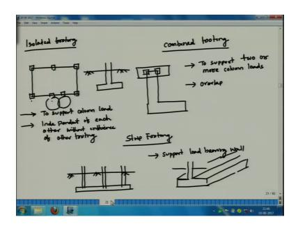
So, then I explain isolated footing where the case and to support your column loads and combined footings.
