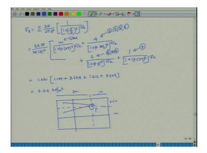
Now, is a sum it of, the summation will be sigma z equal to summation of 3 Q by 2 p I z square in to 1 by 1 plus r by z whole square to the power your 5 by 2. And this comes out to be if I write it 3 in to Q is equal to 22 p I in to z square is equal to 3 whole square in to here it is 1 by 1 plus 0.507 whole square to the power 5 by 2.
