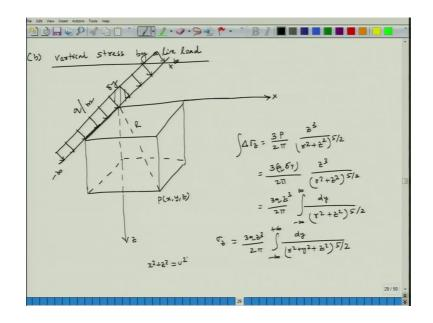
Now, let us come back to this is about your point load. So, vertical stress by a line loads. Second one is your vertical stress by a line load. So, basically it started this derivation is basically from the extended version from your vertical stress below a point load. Let me draw in such a way it will be more you can understand more easily. This will be a z, and this will be a p into x y and z. And this is your x, and now I am taking in these directions.
