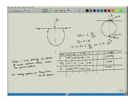
So, we have covered vertical stress distribution; that means isobar then let us start with vertical stress distribution on a horizontal plane.
