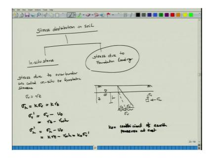
So earlier covered stress distribution in soil last class; in situ stress due to foundation loading.
