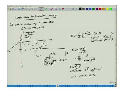
So, in case of stress due to foundation loading it is primarily important for your design of a foundation; that means, increasing stress because of your external loading. So, stress due to foundation loadings stress caused by a point load we have started with boussinesq 1985.
