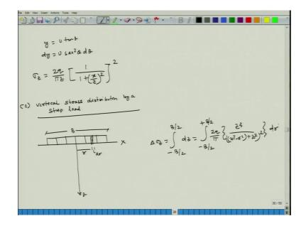
Now, So, if I put it y is equal to u tan theta and dy is equal to u sec square theta d theta, then how it comes out to be in the form of if I solve it is coming out to be sigma z is equal to 2 Q by pi z into 1 by 1 plus x by z hole square here it is a hole square. After solving this equations after solving this equation 2 Q by pi z 1 by 1 plus x by z hole square to the power hole square.
