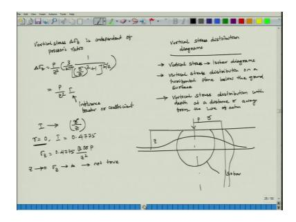
Then vertical stress distribution diagram one is your isobar second is your vertical stress distribution on a horizontal plane below the ground surface. Vertical stress distributions with a depth at a distance are away from the line of action.
