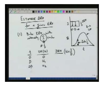
Now if a rainfall of intensity I occur then the DRH ordinate will simply be u into  $I_1$  over D because 1 hour D is the intensity for which we have unit hydrograph and I is the actual intensity of rainfall. So DRH ordinate will be  $0u_1I$  over D,  $u_2I$  over D which is basically the same as this whole curve will shift up or down depending on whether I is more than 1 hour D or less than 1 hour D.
