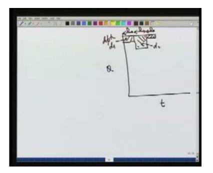
So let us say that this ERH has depth  $d_1$ . This has  $d_2$  and this has depth of  $d_3$  and what we have is we have the measurement of the runoff at the basin station A which looks like this. Now from this measurement of direct runoff hydrograph, what we want to estimate is what will be the unit hydrograph for a D hour duration rainfall and in order to do that we again use the principle of super position. (Refer Slide Time: 53:15)
