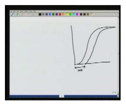
As we have discussed, you can get hydrograph for any other duration by drawing the S curve and shifting it by XD. Now these direct runoff ordinates they are due to storm of intensity 1 over D and period 1XD therefore, the rain, volume or depth of rainfall would be X and therefore in order to compute the unit hydrograph for XD, we will have to divide all these ordinates by X. Now this works well when we have rainfall hydrograph which can be idealized as rainfall of constant
