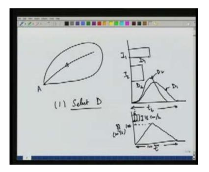
So the area of the rain is 1 cm. The hydrograph is 1 cm. This is the effective depth of rainfall which is falling over the whole catchment. Let us say that area of the catchment is AC and typically these areas are measured in km square.
