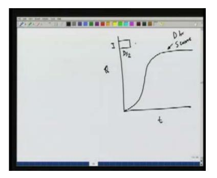
Let us assume that S curve is given by this which represents infinite duration of DRH. What we say is if we lag the ERH by this time D/2, in the first case our ERH starts from 0. In the second case the ERH starts from D/2, then we would get S curve which would be shifted by the amount D/2 and would be parallel to the first S curve.
