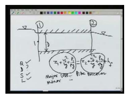
Here this is the culvert and the condition is here, also it is submerged here. We are considering a pipe flow. Let us say this is the diameter, so as usual Q is known D is to be determined and slope
