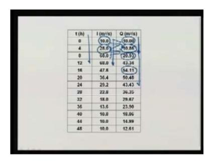
$Q_2$  is obtained from this equation where  $C_0$ ,  $C_1$ ,  $C_2$ .  $I_2$ ,  $I_1$  and  $Q_1$  are obtained from this. For example, in this case  $I_1$  is 10,  $I_2$  is 28 and  $Q_1$  is 10. These 3 values will give us 10.86. When we go to the next step, then we use  $I_1$ ,  $I_2$   $Q_1$ , these 3 values will give us and this way we can proceed with calculating the outflow hydrograph and that is plotted here (Refer Slide Time: 58:21).
