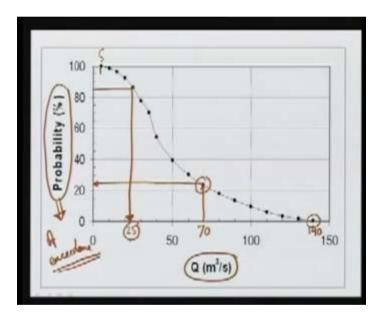
If we design something based on a design value of 25 metre cube per second then it is likely that 85% of the time the discharge will be more than that. This gives us an idea about how much flow is available in a river.
