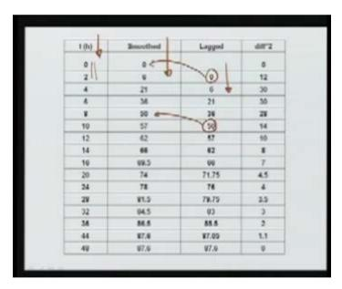
This difference is multiplied by 2 so that we get unit hydrograph for 2 hour duration and this is plotted in this figure. You can see that a 2 hour unit hydrograph is obtained using the S curve; two different S curves one starting from zero, the other lagged and then we take the difference, multiply it by 2 to get the 2 hour unit hydrograph.
