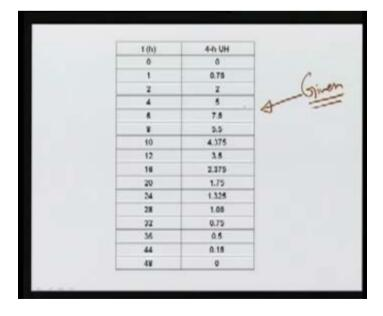
You can look at the ordinates and this is the figure of 4 hour UH. As we have seen already 4 hour UH means this is due to 1 centimetre rain over a period of 4 hours
