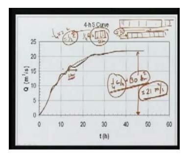
That is what we have done here in the next table. This is time. This is the smooth curve which we have fitted here. The ordinates of that smooth curve are given here and then we lag it by 2 hours. This zero corresponds to this zero with the lag of 2 hours. Similarly this 50 at 10 corresponds to 50 at 8 and so on.
