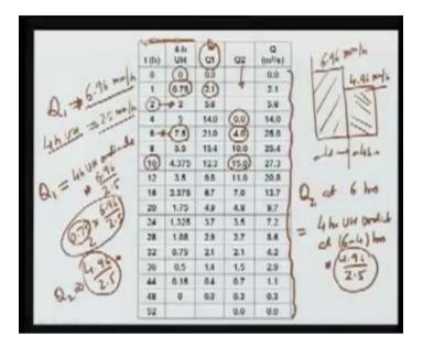
In this way we can superimpose any number of rains provided they are all 4 hour duration and we can plot this. This is from 4 hour; this is the DRH, the solid line shows the value, this value which we have obtained from the 4 hour unit hydrograph and these symbols, this we have shown as the observed from the earlier lessons of measured data at the outlet.
