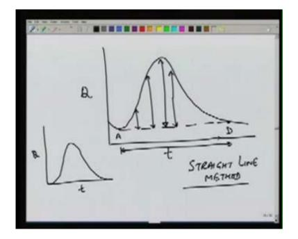
The easiest method is to join A and D with a straight line. Suppose this is the hydrograph, we say that the base flow is given by this line joining A and D and whatever area is above this line, will give the direct runoff ordinate at that time and then we can plot this direct runoff hydrograph separately, which will have a peak equal to this value and a time base which is equal to AD. Time base of course will remain same for all the methods, because we have already fixed the points A and D.
