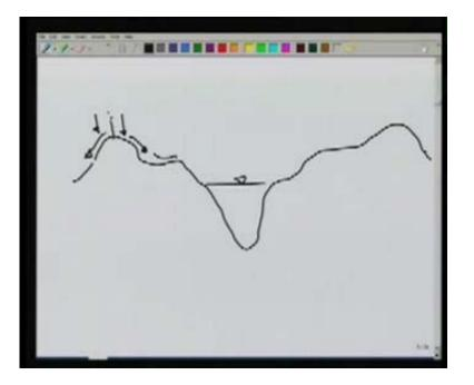
If we look at the elevation, then suppose the ground is like this and this is the river section then any water precipitation falling on this side may come to the river and a precipitation falling on this side may go out of this area. So this will be a water divide, defining the catchment area. Now how do we study the runoff in a river? (Refer Slide Time: 09:47)
