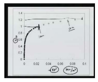
The two curves are quite different here. These two are quite different here but when we make it non-dimensional with respect to r square then we get the same curve and now we can use this single curve for curve matching or the type curve fitting and we can see that the data fits again very well. Here these again are open circles; these are the 50 meter
