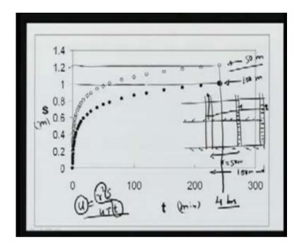
The combined curve shows the same thing. The data for t over r square for 100 meter well stops here which is 1 meter drawdown. The data for the 50 meter curve goes up to 1.2 meter drawdown. t over r square what we are doing is kind of non-dimensionalizing the time with respect to the distance. In t over r square versus S curve S is in meters; t over r square here is minute per meter square.
