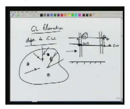
For this case if we have three different observation wells and we have the measurement of ground water elevation and depth to ground water at the three wells we can estimate roughly what is the direction of flow and if we know the hydraulic conductivity, K we can also find out or estimate what is the velocity of ground water movement or if we some how measure the ground water velocity then we can estimate the hydraulic conductivity.
