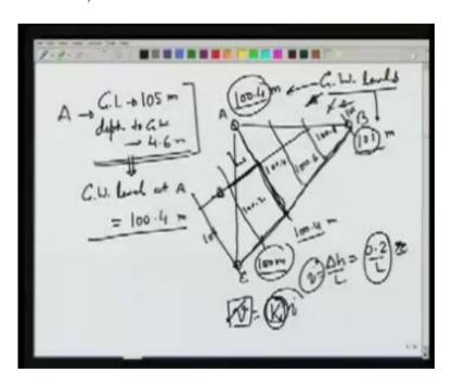
This will give us an estimate of the conductivity if we don't have a pumping well and we have some three observation wells which measure the ground water elevation.
