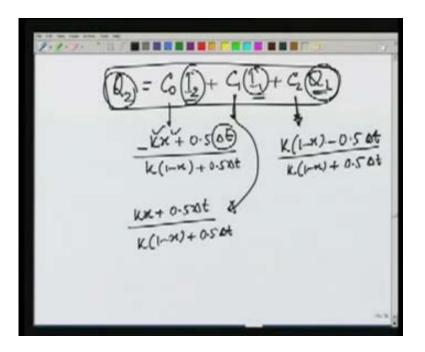
Sometimes it is also written in a different form as Q at any step I .... with previous time step value some constant and delta net inflow before the time step and net inflow after the time step.
