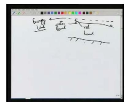
The slope of this line at any point is divided by  $S_f$  and this value of  $S_f$  is obtained from using equations like Manning's equation or Chezy's equation for open channel flow. In this equation  $S_0$  and  $S_f$  are obtained. Bed slope is obtained from geometry of a channel.  $S_f$  is obtained from Manning's or Chezy's equation and then we can solve these two equations together to obtain the value of discharge at all values of x and at different times.
