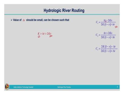
Now, we need to look at the values to be chosen for these  $\Delta t$ , K, x etc. So, the value of  $\Delta t$  should be taken small then only we can assume the flow properties within that time interval to be linear. So, the  $\Delta t$  value is taken in such a way that it is between K and 2Kx, i.e.,
