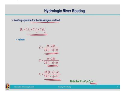
Now, let us look into the routing equation for Muskingum method. The previous equation is put in the simplified form like this  $Q_2$  is a function of  $I_2$ ,  $I_1$ ,  $Q_1$ .  $Q_2$  is written as
