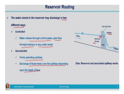
Now, we will move on to the topic of reservoir routing. The water stored in the reservoir may discharge in two different ways, that can be expressed by means of a figure. Here we are having a dam structure and this is the dam and this is representing the top of the dam and reservoir storage is coming in the upstream side of the dam and water flow is taking place above the reservoir. So, that part of the reservoir is having a hydraulic structure, spillway. Spillway is the
