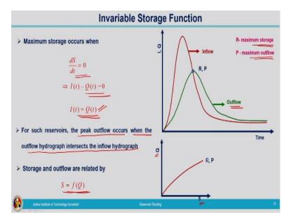
We can look into the properties of the invariable storage function with the help of the hydrographs, that is the inflow and outflow hydrograph, where the maximum storage will be occurring. Mathematically if we are representing, certain quantity is maximum means differential of that particular quantity will be equal to 0. So, here we are going to consider the case with the maximum storage. At the maximum storage,
