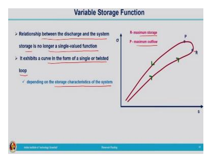
Actually, we want the relationship between the S and Q. Coming to the relationship between the discharge and the system storage is no longer a single valued function. We cannot represent the relationship between the storage and outflow by making use of a single valued function as we have taken in the case of invariable storage function, S = f(Q). It exhibits a curve in the form
