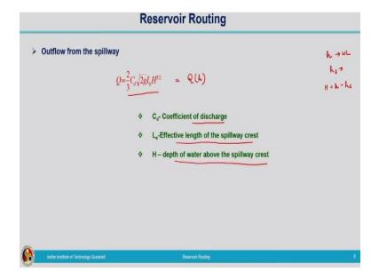
In the case of reservoirs with spillway, outflow from the spillway can be written as
