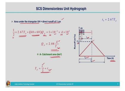
Now, we are going to make use of the principle of unit hydrograph, that is area under the triangular unit hydrograph is equivalent to direct runoff of 1 centimeter, because 1 centimeter of effective rainfall for the particular duration  $t_r$ , that is producing this triangular unit hydrograph, that is our assumption. So, if that is the case, area under the triangular unit hydrograph will be equal to direct runoff of 1 centimeter.
