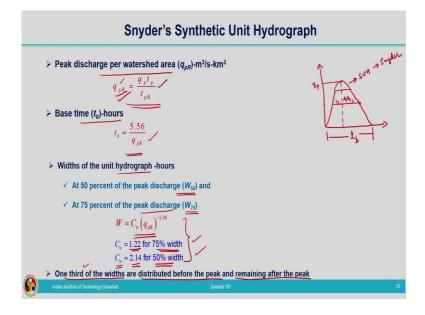
Once  $t_{pR}$  is calculated we can get the values corresponding to peak discharge per watershed area that is  $q_{pR}$  by using this formula,
