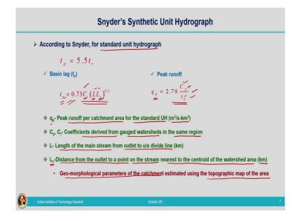
So, now, let us move on to Snyder's method of synthetic unit hydrograph. According to Snyder for standard unit hydrograph
