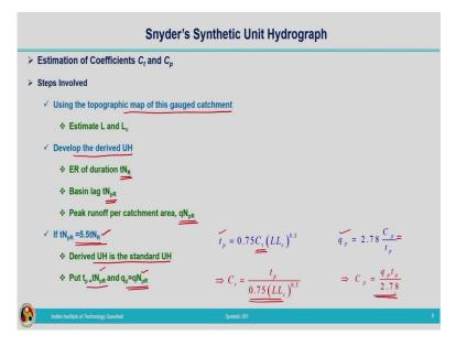
Now, coming to different steps involved in this, using the topographic map of this gauged catchment we can calculate the length such as L and  $L_c$ . After that we can go for developing
