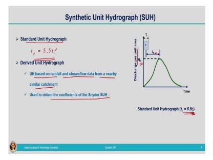
The second terminology related to hydrograph which Snyder has proposed is standard unit hydrograph. Standard unit hydrograph is the one in which
