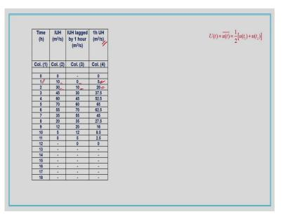
We can move ahead for solving the example. These are the ordinates of IUH given in the question in meter cube per second. How can we determine the unit hydrograph? This we have seen in the lecture related to IUH, from the IUH the unit hydrograph ordinates can be
