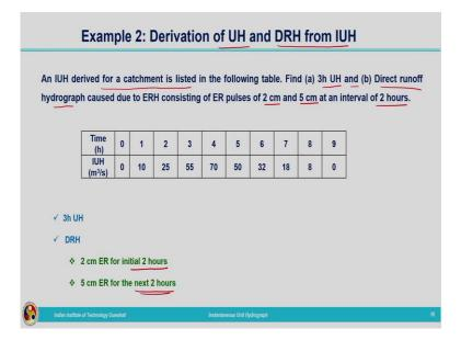
Next example is the derivation of unit hydrograph and direct runoff hydrograph from instantaneous unit hydrograph. Instantaneous unit hydrograph is derived in the previous example. Once instantaneous unit hydrograph is there, we can derive unit hydrograph and also direct runoff hydrograph. So, in this example, we are going to derive the UH and DRH.
