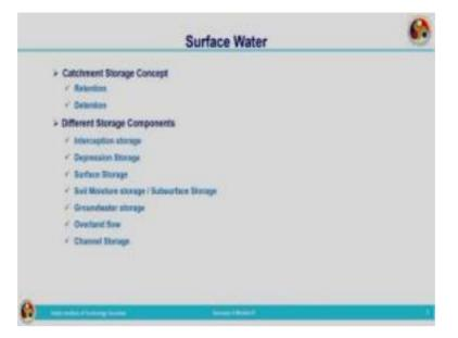
So, this is the general classification of storage. One is the retention and the other one is of detention and again different classification coming under catchment storage components are interception storage, depression storage, surface storage, soil moisture and subsurface storage, groundwater storage, overland flow, channel storage.
