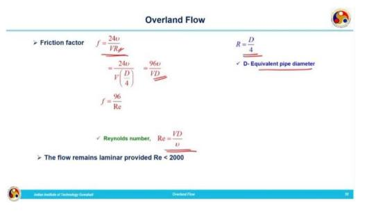
But we know in the case of pipe flow  $R = \frac{D}{4}$ . Hydraulic radius *R* can be written as diameter by 4. This is coming from the expression hydraulic radius is equal to  $\frac{A}{P}$ . Area divided by wetted perimeter and from that we can understand that *R* can be written as diameter divided by 4. So, *D* is the equivalent pipe diameter and here we are substituting for  $R = \frac{D}{4}$ . Then, friction factor *f* will be taking the form
