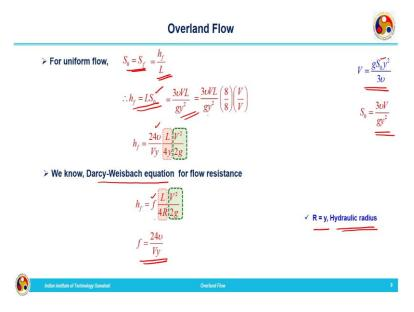
Now, what we are going to do we are going to combine the continuity equation and also momentum equation. For uniform flow we know  $S_0 = S_f$ , that is the bed slope is equal to friction slope, that can be written as  $S_0 = S_f = \frac{h_f}{L}$ .  $h_f$  is the head loss as the flow takes place from one location to another which is having a length of L.  $\frac{h_f}{L}$  will be giving us the slope or the friction slope. So, from that we can write
