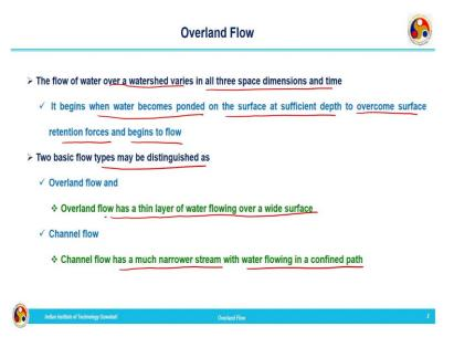
So, in today's lecture we will move on to overland flow. So, the flow of water over watershed varies in all the three dimensions. So, it is a three-dimensional phenomenon, in all the direction the flow of water on the surface of the earth will be taking place. It begins when water becomes ponded on the surface at sufficient depth to overcome surface retention forces and then begins to flow. That is whenever there is a storm or rainfall is occurring, we are
