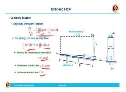
This is the same representation which I have shown in the previous slide. Now, we need to write the continuity equation, when we are going to write the continuity equation, we will be making use of Reynolds Transport Theorem which is given by this equation,
