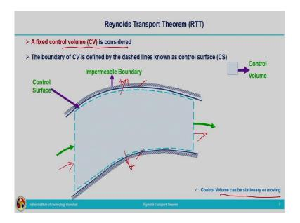
Now, let us move on to Reynolds transport theorem. Reynolds transport theorem is based on Eulerian approach. And here what we are doing? We are going to consider a fluid flow. We can have the pictorial representation of the fluid flow within this domain. So, you can see the flow is taking place within this domain and we are going to consider 2 sections, section 1 and section 2. The fluid flow is taking from left to right.
