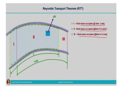
Now, what we are going to do? We are going to consider the control volume for the time t and as we know control volume is not going to change as time changes. So, for the time t, we are having the control volume and also, we are considering the system, that is the control mass. So, a system is marked by the yellow dotted lines which is coinciding with the control volume. System at time t is marked by this yellow dotted line.
