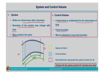
Again, I am coming to system and control volume concept. So, system refers to a fixed mass within a boundary. The boundary of the system may change with time, that is the system is moving from one location to another location as time changes. It is not stationary; it is moving from one location to another location. Thus, in the case of system mass remains the same.
