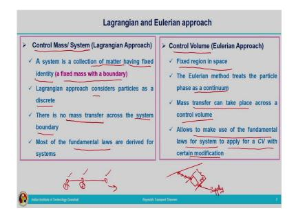
So, first let us see again in detail what is meant by Lagrangian approach and Eulerian approach? So, one thing is that control mass or system and second one is the control volume. So, if we are talking about the fluid flow, we can analyze the fluid flow by making use of Lagrangian approach and Eulerian approach.
