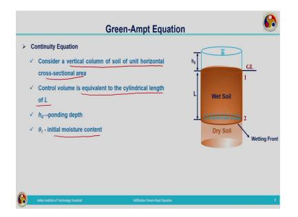
Now we are going to derive the fundamental equations, that is, the mass conservation equation and the momentum conservation equation based on control volume approach. So, for that, we need to consider the control volume. So, take a control volume, below the ground surface within the depth of infiltration water.
