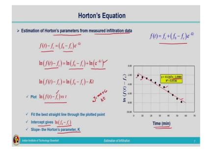
Now let us move on to finding out the Horton's parameters, from the measured infiltration data. This is our Horton's infiltration rate equation. So here, some rearrangements of the terms, which are present in the equation, will be done. So, we are writing
