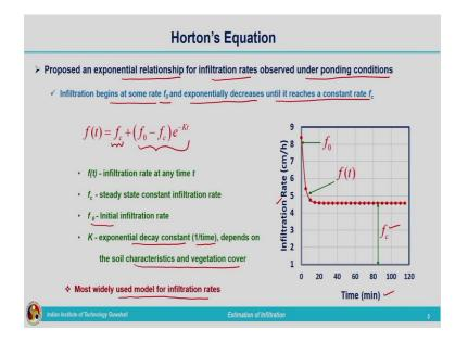
Next equation is Horton's Equation. This equation is also very commonly used for finding out the infiltration rate and cumulative infiltration, but we should be aware of the parameters corresponding to Horton's equation. So, let us see how this equation is looking like. This is proposing an exponential relationship for infiltration rates observed under ponding condition.
