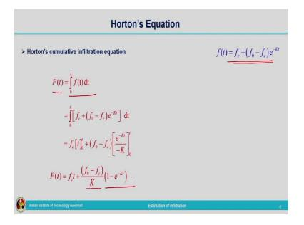
Relationship between the infiltration rate and cumulative infiltration is known to us. Just integrating the infiltration rate curve will be giving us the cumulative infiltration.
