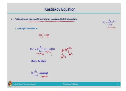
Now, this equation is having two coefficients,  $K_k$  and  $\alpha$ . So, these coefficients need to be determined. So next, let us see estimation of two coefficients from the measured infiltration data. This is our equation.
