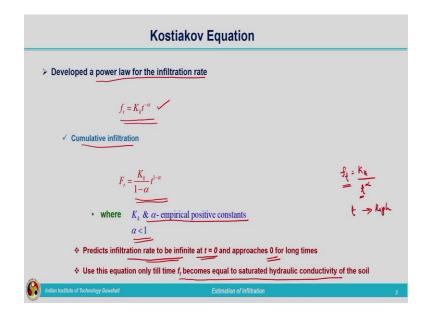
First one is the Kostiakov equation. In this, a relationship is developed as a power law for the infiltration rate. So, infiltration rate is expressed by means of a power law. The equation is given by
