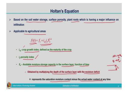
Now next equation is Holtan's Equation. In Holtan's Equation, some more factors are taken into account. It is based on the soil water storage, surface porosity, and plant roots, which is having major influence on infiltration. If plant roots are more, it will be creating some extra pores, macropores within the soil that will be aggravating the infiltration rate. So that is also taken into account while deriving Holtan's Equation.
