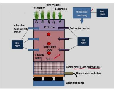
Let us see an engineered Lysimeter, this is a tank which can be used as a Lysimeter. So, bottom layer we are having the coarse gravel or sand drainage layer. So, we are not completely filling the tank with soil, it will be having different layers, bottom layer is fixed for draining of the water. So, in this region we will be filling the coarse gravel or sand. Above that, we will be filling the soil and upper part is the root zone and will be growing different plants.
