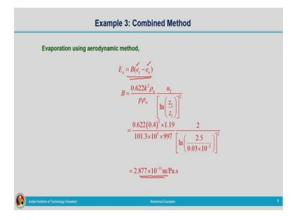
Now, the second approach is the aerodynamic method. By using the aerodynamic method, evaporation can be calculated by using this formula
