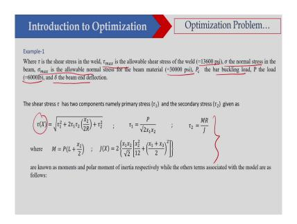
So, this problem has this particular details. So, where tau is the shear stress and tau max is the allowable shear stress and this value is given and sigma is the normal stress and sigma max is the allowable normal stress that also given and P c is the bar buckling load and the bar buckling load is given here ok.
