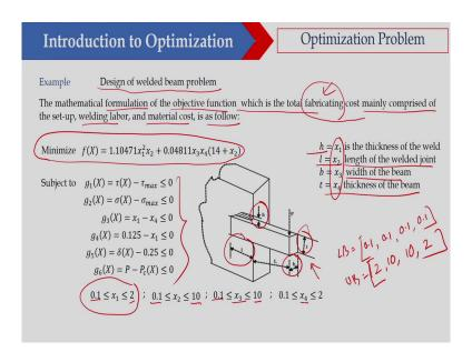
So, this is the problem. So, this problem is design of welded beam. So, design of a welded beam. So, this is the welded beam here I have shown in this particular figure. So, this is the figure and I would like to design this welding ok. The mathematical formulation of the objective function which is the total fabrication cost ok.
