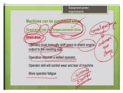
So, another important thing to be noted is the machines when you purchase depending upon the mode of transmission, you can call it as direct drive base machine or torque converted drive-based machine. In a simple way to say it is nothing but your manual gear change versus automatic gear change. So, basically your direct drive is nothing but your manual gear change.
