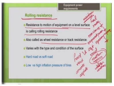
The first thing we will discuss about the rolling resistance. Rolling resistance is nothing but what is the resistance offered by the hauled route to the wheel which is rolling over the particular surface. So, what is the resistance offered by the hauled route to the wheel which is rolling over the particular surface, so that is what is your rolling resistance. So, resistance to the motion of equipment on a level surface is called as rolling resistance.
