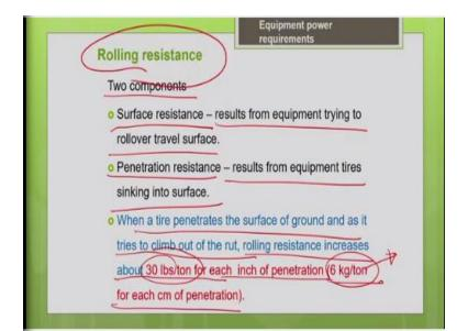
So, what are all the 2 important components of the rolling resistance? Let us see, one is the surface resistance other one is your penetration resistance. So, you can break this rolling resistance into 2 components, one is at the surface. So, the resistance which is encountered at the surface when the; wheel is moving over or rolling over the surface that is surface resistance.
