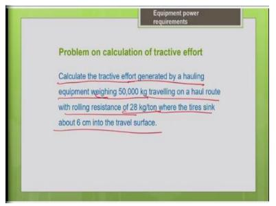
Now, for better understanding, let us work out a problem on calculation of the tractive effort. So, calculate the tractive effort generated by a hauling equipment, it is gross weight is given as 50,000 kg, it is traveling on a haul route. It is rolling resistance is given to you directly you can take it from the literature for that particular haul route; it is given as 28 kg per ton. And another important thing to be noted is your tire is sinking about 6 centimeters into the travel surface.
