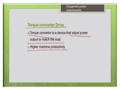
So, other one as we discuss just now is torque converter drive, it is initial cost is high. So, you have a torque converter device here which can automatically match your adjust your power output to match the load conditions, so it results in higher productivity. So, you know why higher productivity because your maneuver time is going to be lesser here, your cycle time will be reduced, so the productivity will increase.
