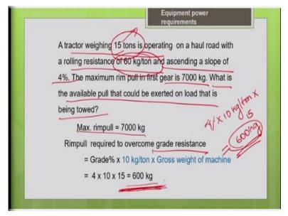
Now let us workout the problem on how to estimate the power requirements of the machine. So, a tractor weighing 15 tons is operating on a haul road, the gross weight of the machine is given as 15 tons. It means it includes it is empty weight as well as the load it is carrying, with the rolling resistance of 60 kg per ton, it is given you can take it from the literature also for this particular haul route.
