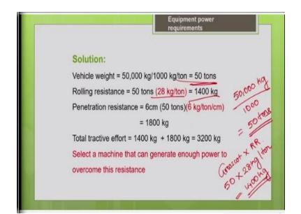
So, let us convert the vehicle weight into tons, because your rolling resistance is commonly expressed as kg per ton. So, let us convert the weight of the machine into tons you know that the gross weight of the machine is given as 50,000 kg. So, 1000 kg = 1 ton, so divided you will get the gross weight of the machine as 50 tons. Now the rolling resistance you need to calculate for this particular haul route it is given as 28 kg per ton.
