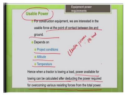
So, where a tractor is towing to load, the power available for towing can be calculated after detecting the power required for overcoming the various resistance forces from the total power. So, this we have to keep in mind, so this is nothing but your usable power.
