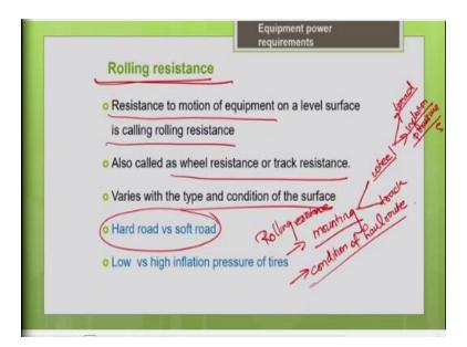
As I told you, it varies a lot with the type and the condition of the surface. And also, it depends upon the mountin, it depends upon the condition of your surface, condition of your hauled route. So, mounting in the sense, it can be either a wheel mounted or it can be a track mounted. If it is wheel mounted, even your dimension of your tyre, the tread dimension of your tyre and the inflation pressure of your tyre, all these things are going to affect your rolling resistance.
