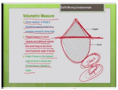
So, first is the struck measure. See, basically say for example, you have the bucket of your excavator, so you are going to excavate the load, you are going to load the bucket of your excavator, how do you express the volume of the bucket? See basically, there are different ways to express the volume; either you can express it on the basis of struck capacity or heaped capacity.
