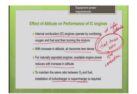
Now let us see what is the effect of altitude on the performance of the engine? So, as we discussed earlier, the usable power depends upon the underfoot conditions, altitude and temperature. So, you know that the horsepower rating of the machine is done with the standard conditions by the manufacturer. So, they might have done the horsepower rating at standard temperature and the standard atmospheric pressure.
