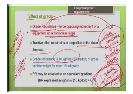
Grade resistance is nothing but by simple elementary I mean a mechanics people have worked out this the relations. Say for example, for 1% of grade so the amount of tractive effort needed to overcome this 1% of grade it is 10 kg per ton. So, this is simple guideline which they are worked out which is worked out in the literature you can easily find it. So, for 1% of grade, so the grade resistance is 10 kg per ton.
