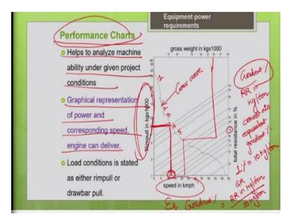
So, you have to draw a vertical line intersecting your total resistance percentage line. Once it intersects your; the total resistance percentage line, then draw a horizontal line to the left intersecting your gear curve. Now drop a vertical line intersecting your speed, so this is how you can find the speed of the machine if you know the total resistance percentage.
