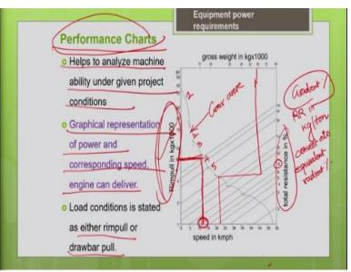
So, either you can use this rimpull in kg and find the speed or you can use the total resistance in percentage and you can use the gross weight and find the actual speed of the machine possible for this particular project condition. So, depending upon the mounting your low condition can be stated either in the rimpull or in the draw pull. So, depending upon the whether it is tyre mounted machine or track mounted machine accordingly.
