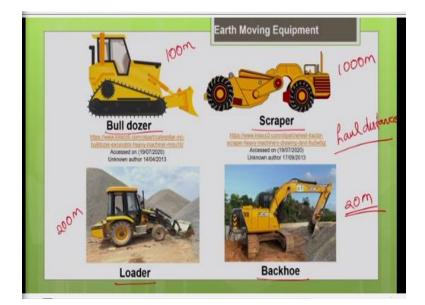
So, let us look into what all are the earthmoving equipment which are commonly used for the earthmoving operations. So, you can see this bulldozer, this is a scraper, this is the loader, front end loader and this is a backhoe, we call this an excavator. So, basically which equipment we need to select depends upon your project requirements. We have discussed about the factors influencing the selection of the equipment in the lecture 1, hope you remember.
