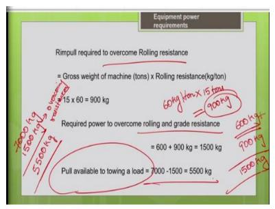
Now let us calculate how to estimate a tractive effort to overcome the rolling resistance? So, it is nothing but for this particular haul route the rolling resistance value is given us 60 kg per ton. So, what is the gross weight of your machine? It is nothing but 15 tons. So, that gives me the total
