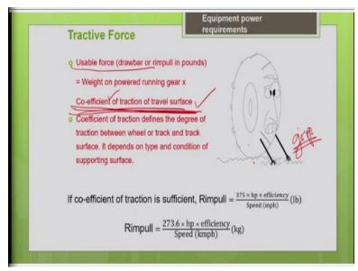
So, how to calculate this usable force? So, this usable force is going to depend upon the traction of your travel surface. So, as I told you how much amount of the total power becomes usable, it depends upon the degree of traction between your wheel and the ground. Traction is nothing but
