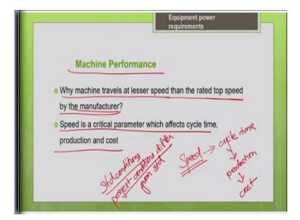
So, there are some more important terms you need to learn with respect to the machine performance. Basically, speed is a very important parameter used to quantify the machine performance. Most of the contractors are interested in the speed of the particular equipment. Because speed will affect your cycle time of the machine that is going to affect your production of the machine, that is going to in turn affect the cost associated with the machine.
