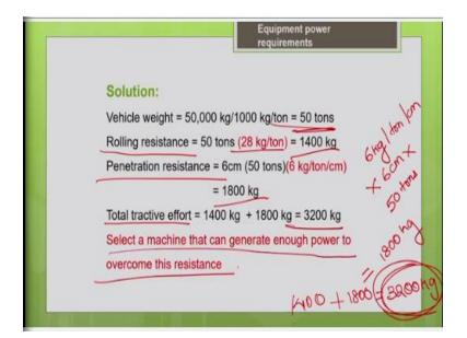
So, you multiply that by how much is the depth of penetration? It is nothing but 6 centimeter, and what is the gross weight of the machine? It is nothing but 50 tons. So, that gives you the penetration resistance as 1800 kg. Now we can find the total resistance, that is nothing but add your rolling resistance and the penetration resistance. It is nothing but your 1400 kg + 1800 kg, so that gives me the answer as 3200 kg is the total resistance.
